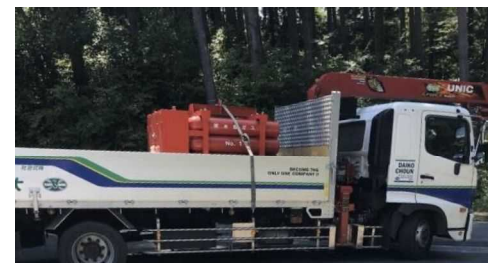
Cylinders are transported in a bundle to local demands by trucks.
